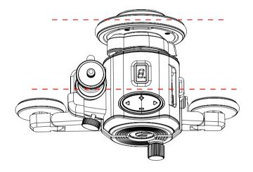
For straight movement keep wheels aligned parallel
