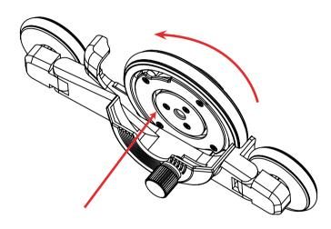
Rotate the wheel to lock into place
