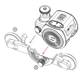
Place the Movie Maker into the Micro Dolly cradle base and fasten using the fastening screw
