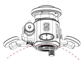
Adjust wheel angle for desired curved movement
