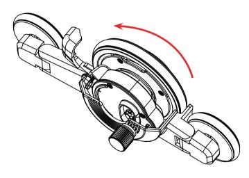
Rotate Power Wheel to lock into place.
